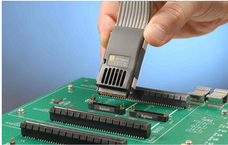
Figure 8 N5345A soft touch probe aligned over back plane
