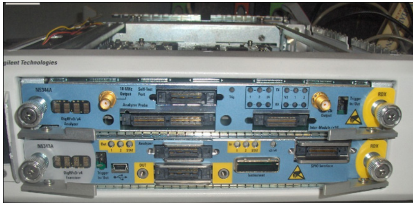
Figure 1 Modules in N5302A chassis
