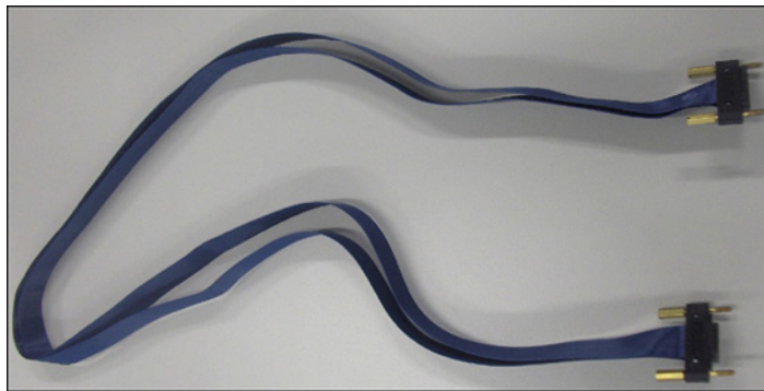
Figure 5 GPIO Bus Cable
